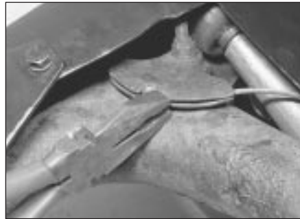
10.10 Pinching the ends of the moving sector to retain the handbrake cable
