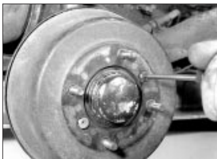
4.2c Remove the brake drum retaining screws . . .
