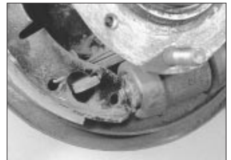
5.7c . . . and rear shoe from the handbrake lever and wheel cylinder
