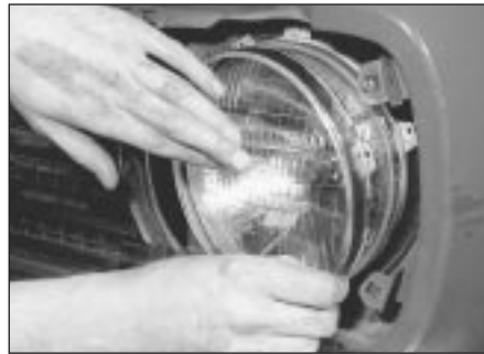
5.4b . . . and lift off the inner rim
