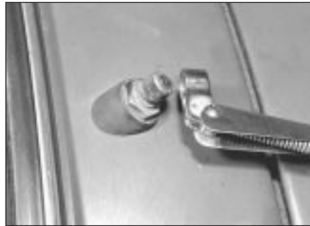
10.2 The wiper arm is a push fit on the wiper spindle splines
