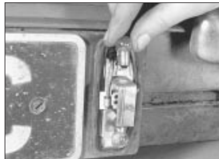
5.48 . . . and remove the bulbs by turning them anti-clockwise
