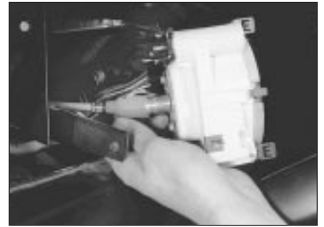
15.28a Detach the speedometer cable ...
